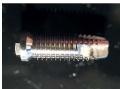
Machined SurfLink dental implant.
