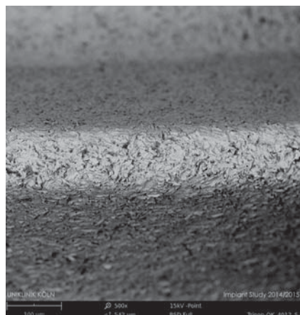
31 | Upper thread, QK implant, Trinon (x500).
